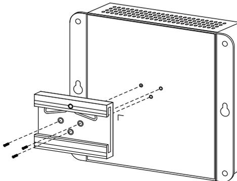
**Step 2:** Lightly insert the bottom of DIN-rail into the track.
